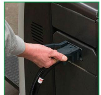
The OTP can be equipped with different tow pins to fit most of the existing trailer equipment on the market. Choose between a manual or automatic tow-hitch with an ergonomic release handle. Connectors and different electric and hydraulic power solutions for active load carriers are also available.
